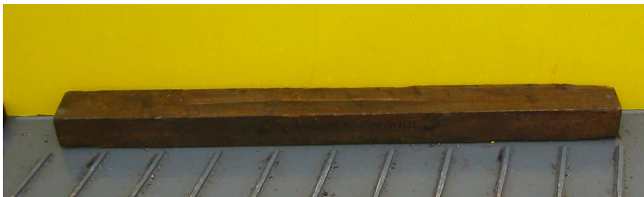
Wooden block to secure trucks in the ramp area on inland-waterway ships
